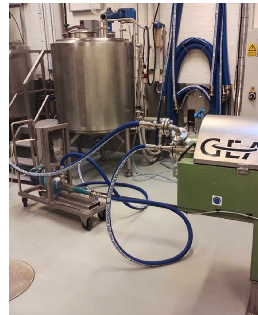
Tank and decanter centrifuge in the Danish pilot
